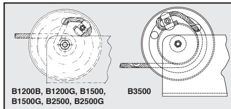
**WINCH MAINTENANCE** — Keep winch in good working order. Damaged or severely-worn parts create unnecessary dangers and could result in personal injury or property damage. The winch requires periodic maintenance. The following check should be made at least once annually and more frequently when the winch is exposed to an environment which is particularly dirty or wet.
