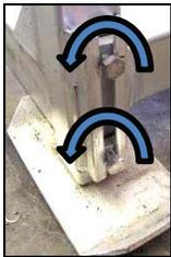
**Step 1** – Loosen (but do not remove) the bolts on the front 2 leg brackets with a 3/4” or 19mm wrench. This will allow the leg posts to move freely.
