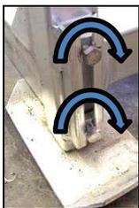
**Step 3** – Tighten both bolts on the front 2 leg brackets with a 3/4” or 19mm wrench.
